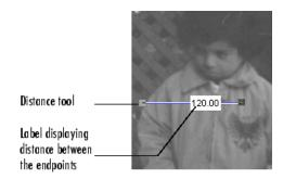
You can move the Distance tool over an image by dragging it with the mouse. You can also resize the Distance tool by selecting one of the endpoints with the mouse and dragging the endpoint.
