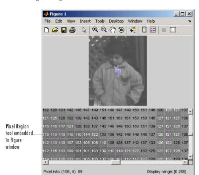
The following figure shows the Pixel Region embedded in the same figure as the target image.
