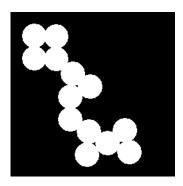
**2** Create a disk-shaped structuring element. Use a disk structuring element to preserve the circular nature of the object. Specify a radius of 10 pixels so that the largest gap gets filled.
