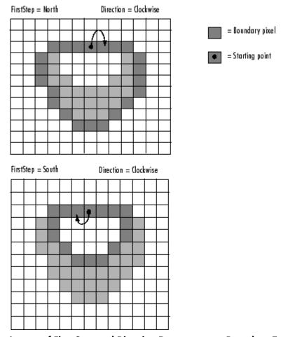
Impact of First Step and Direction Parameters on Boundary Tracing
