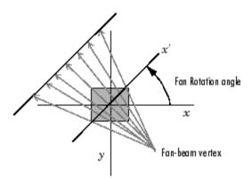
'FanSensorSpacing' -- Positive real scalar specifying the spacing of the fan-beam sensors. Interpretation of the value depends on the setting of 'FanSensorGeometry'. If 'FanSensorGeometry' is set to 'arc' (the default), the value defines the angular spacing in degrees. Default value is 1. If 'FanSensorGeometry' is 'line', the value specifies the linear spacing. Default value is 1.
