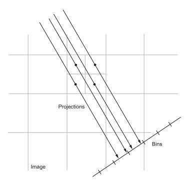
Each subpixel's contribution is proportionally split into the two nearest bins, according to the distance between the projected location and the bin centers. If the subpixel projection hits the center point of a bin, the bin on the axes gets the full value of the subpixel, or one-fourth the value of the pixel. If the subpixel projection hits the border between two bins, the subpixel value is split evenly between the bins.
