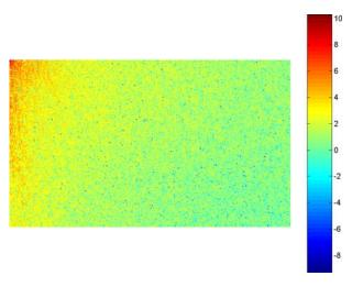
Now set values less than magnitude 10 in the DCT matrix to zero, and then reconstruct the image using the inverse DCT function idct2.
