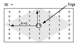
SE = strel('disk', R, N) creates a flat, disk-shaped structuring element, where R specifies the radius. R must be a nonnegative integer. N must be 0, 4, 6, or 8. When N is greater than 0, the disk-shaped structuring element is approximated by a sequence of N periodic-line structuring elements. When N equals 0, no approximation is used, and the structuring element members consist of all pixels whose centers are no greater than R away from the origin. If N is not specified, the default value is 4.
