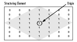
Origin of a Diamond-Shaped Structuring Element
