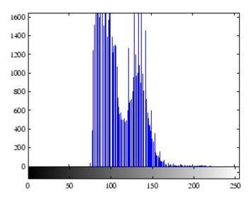
Notice how the intensity range is rather narrow. It does not cover the potential range of [0, 255], and is missing the high and low values that would result in good contrast.
