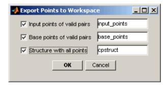
This option saves the positions of all the control points you specified and their current states in a cpstruct structure.
