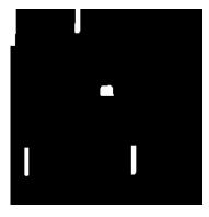
**4** To restore the rectangles to their original sizes, dilate the eroded image using the same structuring element, SE.
