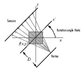
Fan-Beam Projection at Rotation Angle Theta
