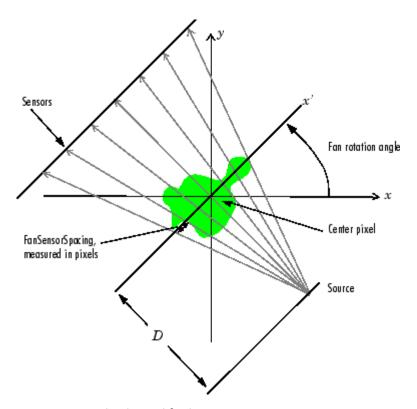
Fan-Beam Projection with Line Geometry
