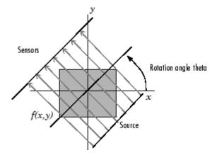
Parallel-Beam Projection at Rotation Angle Theta
