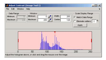
**Note** The Adjust Contrast tool can handle grayscale images of class double and single with data ranges beyond the default display range, which is [0 1]. For these images, imcontrast sets the histogram limits to fit the image data range, with padding at the upper and lower bounds.
