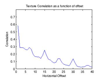
The plot contains peaks at offsets 7, 15, 23, and 30. If you examine the input image closely, you can see that certain vertical elements in the image have a periodic pattern that repeats every seven pixels. The following figure shows the upper left corner of the image and points out where this pattern occurs.
