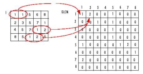
glcms = graycomatrix(I, param1, val1, param2, val2,...) returns one or more gray-level co-occurrence matrices, depending on the values of the optional parameter/value pairs. Parameter names can be abbreviated, and case does not matter.
