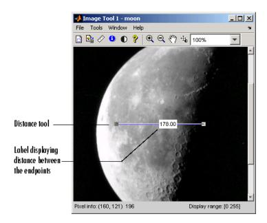
**3** Using the mouse, you can move the Distance tool over the image or, by grabbing either one of its endpoints, resize the tool.
