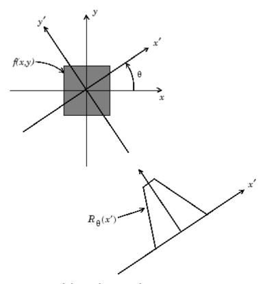
**Geometry of the Radon Transform**
