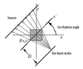
Each column of F contains the fan-beam sensor samples at one rotation angle. The number of columns in F is determined by the fan rotation increment. By default, the fan rotation increment is 1 degree so F has 360 columns.
