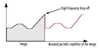
This high-frequency drop-off can create an effect called boundary related ringing in deblurred images. In this figure, note the horizontal and vertical patterns in the image.
