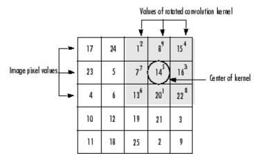
Computing the (2,4) Output of Convolution
