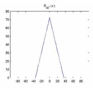
Radon Transform of a Square Function at 45 Degrees
