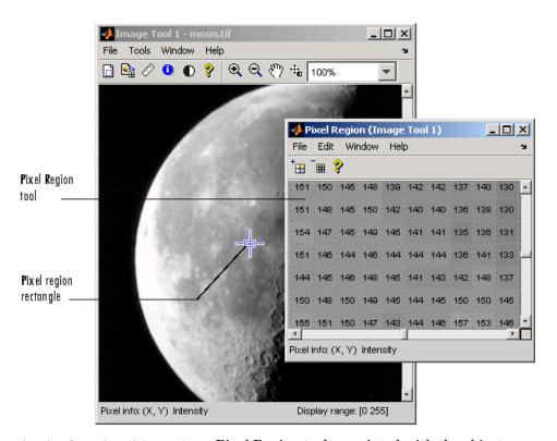
impixelregion(h) creates a Pixel Region tool associated with the object specified by the handle h. h can be a handle to a figure, axes, uipanel, or image object. If h is a handle to an axes or figure, impixelregion associates the tool with the first image found in the axes or figure.
