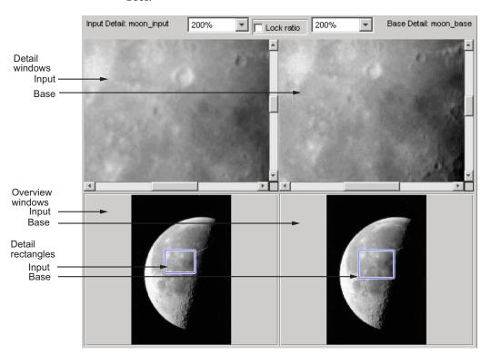
The following figure shows these components of the Control Point Selection Tool.
