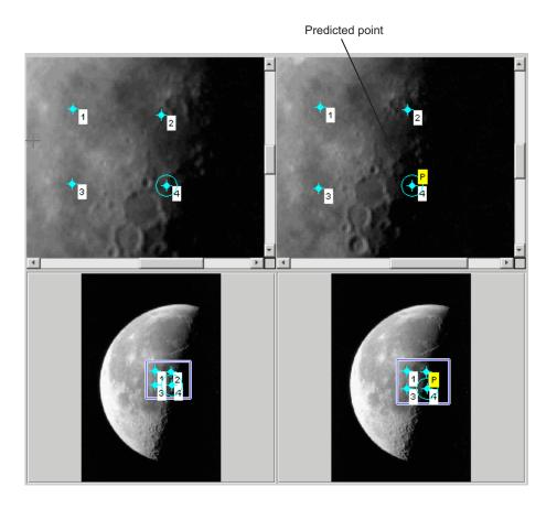
**Note** By default, the Control Point Selection Tool does not include predicted points in the set of valid control points returned in input\_points or base\_points. To include predicted points, you must accept them by selecting the points and fine-tuning their position with the cursor. When you move a predicted point, the Control Point Selection Tool changes the symbol to indicate that it has changed to a standard control point. For more information, see "Moving Control Points" on page 7-25.
