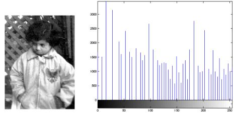
Image After Histogram Equalization with Its Histogram
