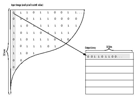
Binary image packing is used to accelerate some binary morphological operations, such as dilation and erosion. If the input to imdilate or imerode is a packed binary image, the functions use a specialized routine to perform the operation faster.
