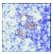
**4** Use deconvreg to deblur the image, specifying the PSF used to create the blur and the noise power, NP.
