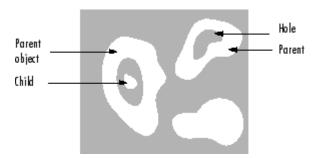
bwboundaries returns B, a P-by-1 cell array, where P is the number of objects and holes. Each cell in the cell array contains a Q-by-2 matrix. Each row in the matrix contains the row and column coordinates of a boundary pixel. Q is the number of boundary pixels for the corresponding region.
