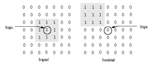
Dilating with a translated version of strel(1) is a way to translate an input image in space by an integer number of pixels. This example translates the cameraman.tif image down and to the right by 25 pixels.
