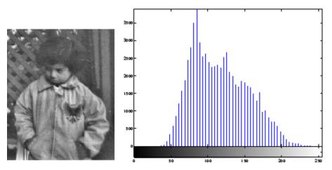
Image After CLAHE Equalization with Its Histogram
