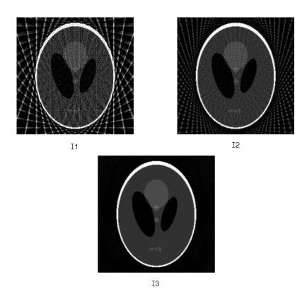
Inverse Radon Transforms of the Shepp-Logan Head Phantom
