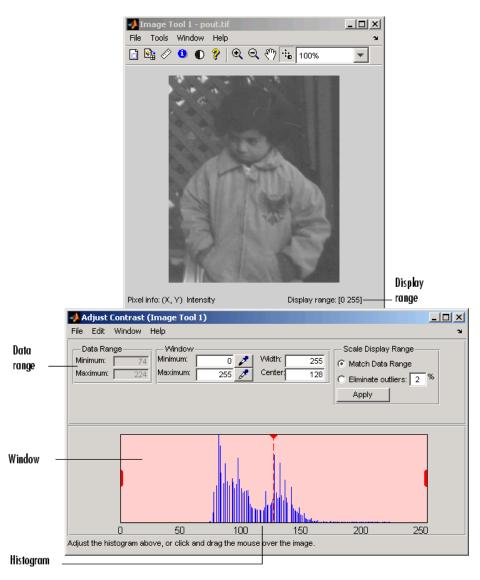
Image Tool with Adjust Contrast Tool
