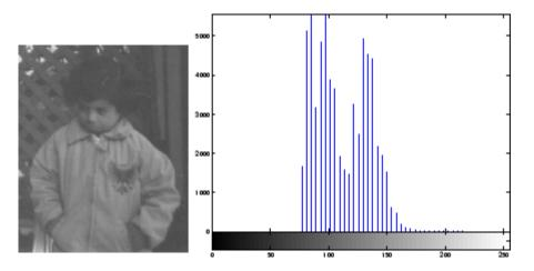
If you remap the data values to fill the entire intensity range [0, 255], you can increase the contrast of the image. The following sections describe several intensity adjustment techniques, including
